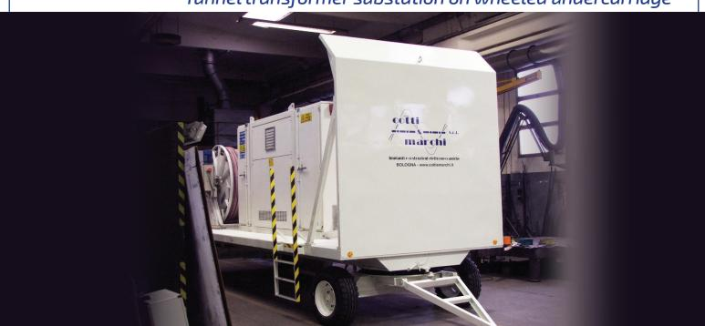
**TUNNEL TRANSFORMER SUBSTATION ON WHEELED UNDERCARRIAGE**, when the tunnel transformer substation opertaes on uniform grounds can be provided with MV/LV cable reel and located on a wheeled undercarriageundercarriagetensione.
